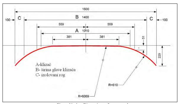
Figure No 1. – Dimensions of pantograph
