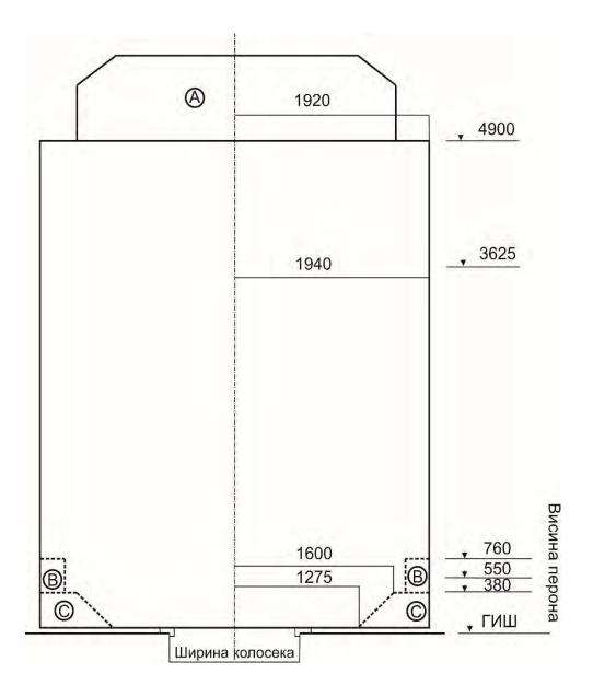
A – Pantograph movement space
